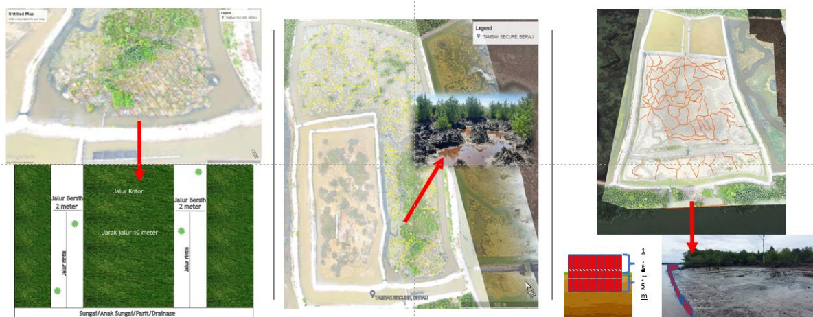
Picture 3. Designs of mangrove restoration to allow for natural mangrove regeneration
